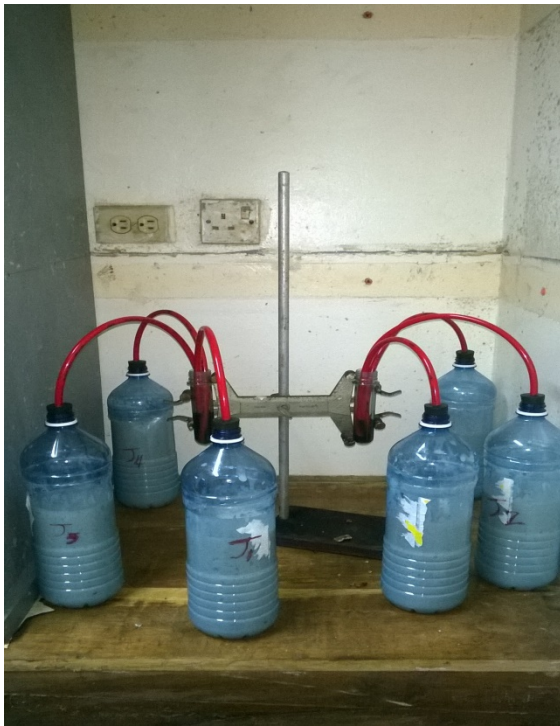
Fig. 2.0 (a) above shows how apparatus that was set up to conduct fermentation, whereas Fig. 2.0 (b) is the apparatus used for distillation.
