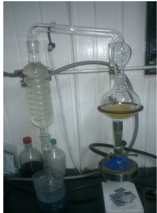
Fig. 2.0 (a) above shows how apparatus that was set up to conduct fermentation, whereas Fig. 2.0 (b) is the apparatus used for distillation.
