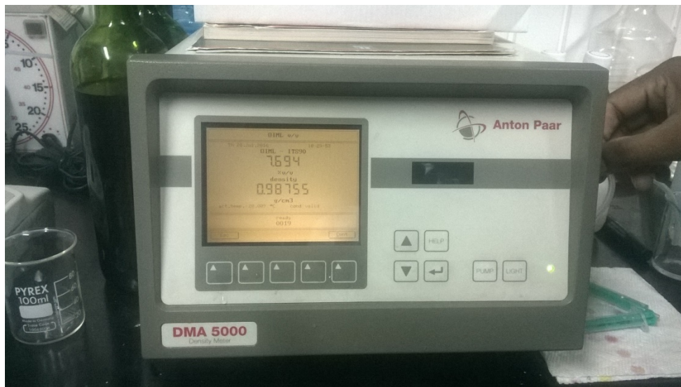
Figure 3.0 shows the Density Meter used to determine Brix and % ethanol.
