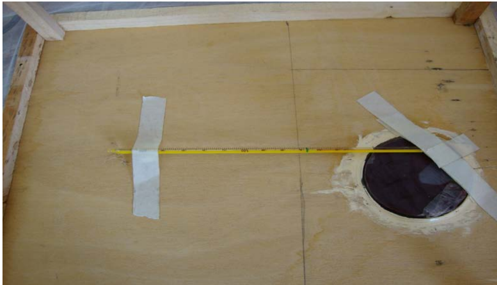
Figure (2): Petri Dish Contain Cotton Soaked with Blood Covered with Parafilm, to it a Thermostat was Attached.
