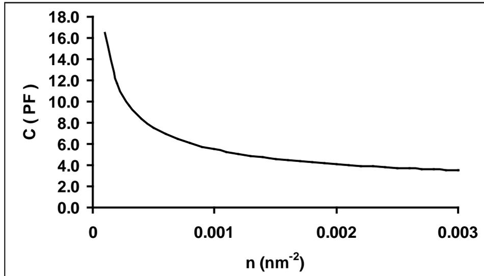
Fig.2 Capacitance as a function of electron area density.
