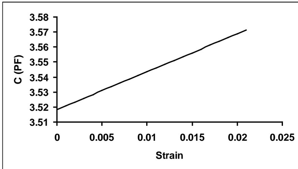
Fig.3 Capacitance as a function of strain.
